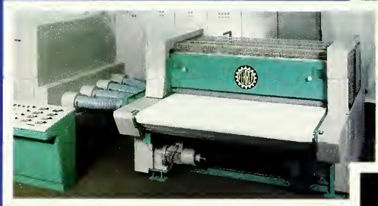
FEHRER K-21 RANDOM CARDING MACHINE has weight range 10-200 g/m 2 , production speed 50-150 m/min.
